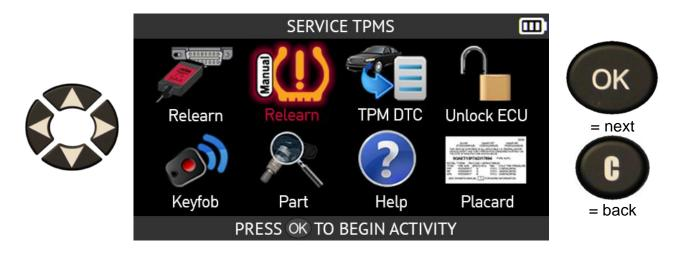
Follow the **RELEARN PROCEDURE** instructions 1/12•Set tyre pressure on screen to 2/12•Engage Parking Brake OK put the 3/12•Turn the ignition to OFF position then press and vehicle into relearn release the brake pedal = next mode. 4/12•Quickly turn the ignition from OFF to RUN (engine OFF) 3 times (stop in RUN position) L Select 5/12•Press and release the brake pedal NEXT 6/12•Set the ignition to OFF = back to read the NEXT, PRESS OK rest.
