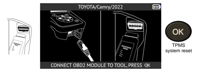
When the vehicle's TPMS system has been reset, the tool will return to the **TPMS service** screen.
