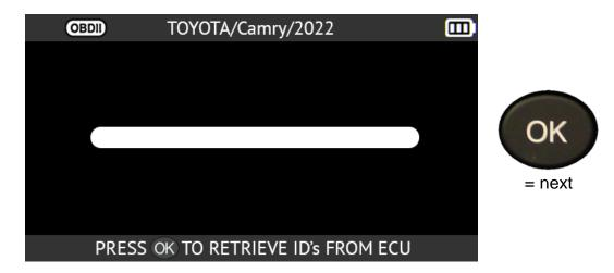
The tool will connect to the vehicle's ECU.
