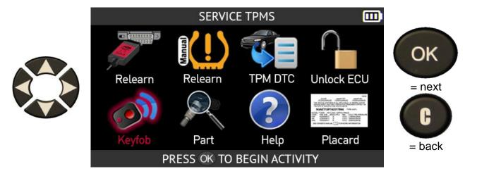
Depending on the make and model of the selected vehicle, the tool will ask you to choose the communication frequency for the key fob being tested.
