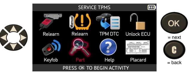
Use the arrow buttons to select the type of spare part you are looking for in the database.
