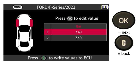
Use the up arrow button to increase the reference pressure value of the selected wheels and the down arrow button to decrease the value.
