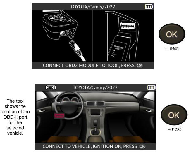
Connect the OBD-II module to the vehicle then press **OK**.
