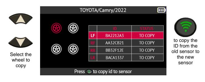
Position the first new sensor in above of the tool's antenna to program it
