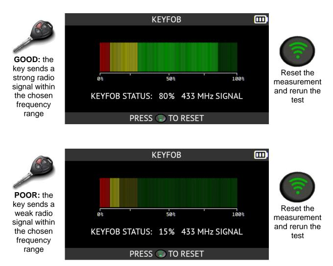
A weak radio signal indicates a low or dead battery. It is recommended that you replace the battery.
