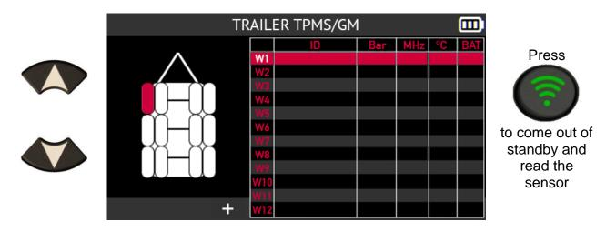
The tool brings the trailer's first sensor out of standby and reads the information it contains.
