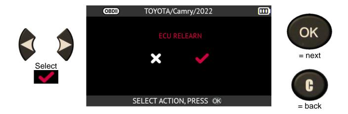
Please note: leave the engine switched off while keeping the ignition switched on.
