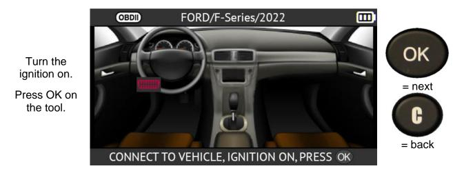
The tool will read the vehicle's reference TPMS data from the ECU.
