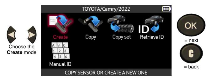
Position the sensor above of the tool's antenna to program it.
