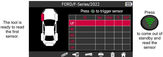
Read each sensor in the order listed in the instructions. Once the last sensor has been read. the horn will honk twice, indicating the relearn has been performed
