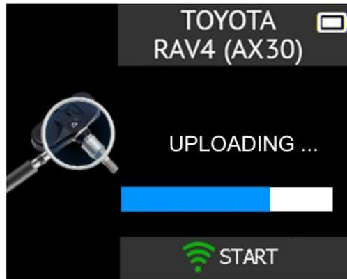
The data has been successfully uploaded to the sensor.
