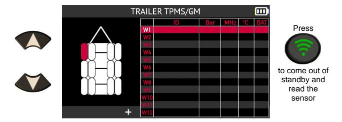
The tool brings the trailer's first sensor out of standby and reads the information it contains.
