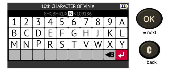
The tool indicates the model year of the vehicle. Press **OK** to move on to the next step.
