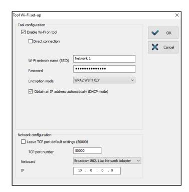
You can check that the tool is properly connected to the WebVT software via WiFi at any time. To do this, select **WiFi set-up** from the menu bar.
