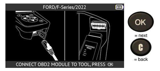
Connect the OBD-II module to the vehicle's OBD port.
