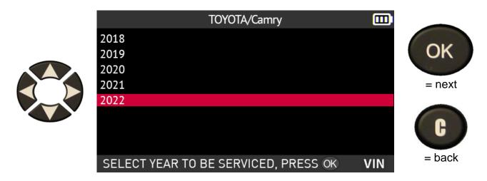
If the year in which the vehicle was put into service is unknown, select the **VIN** icon in the lower right-hand corner of the screen using the arrow buttons. Press **OK** to confirm your choice.
