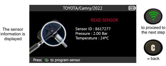
Position the new sensor in above the tool's antenna to carry out the programming.
