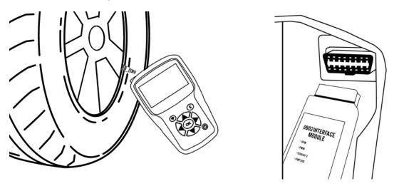
Please note: When the vehicle is in "learn mode" some vehicles will confirm that the sensor information has been communicated with the TPMS system through a series of beeps.
