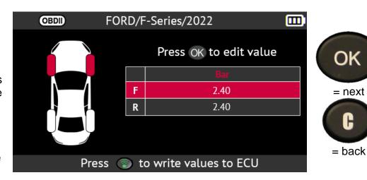
Use the up arrow button to increase the reference pressure value of the selected wheels and the down arrow button to decrease the value.
