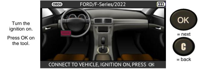
The tool will read the vehicle's reference TPMS data from the ECU.
