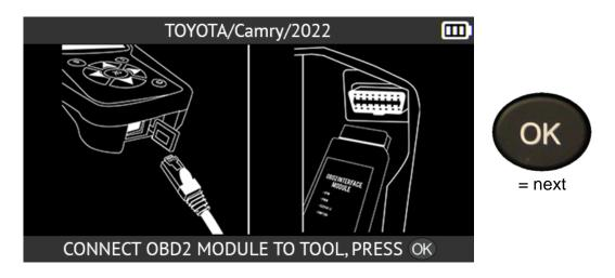
The tool shows the location of the OBD-II port for the selected vehicle.
